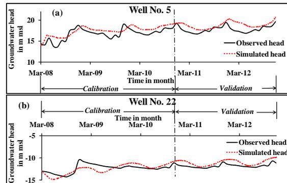
**Figure 8** Temporal variation in observed and simulated groundwater head for (a) well no.5 in upper aquifer and (b) well no.22 in lower aquifer
