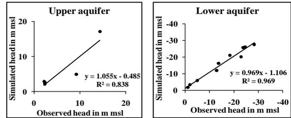
**Figure 6** Steady state calibration in upper and lower aquifer
