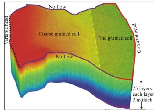
Figure 5 Three dimensional discretization of the study region for modelling
