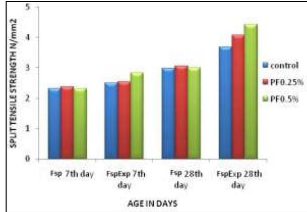
Figure 6: Split tensile strength of PFRC at various ages
