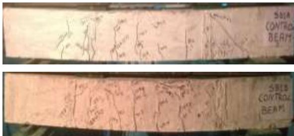
Figure 10: Crack pattern of control beams
