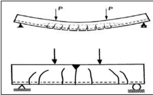
Figure 13: Teeth formation and flexural failure [15]
