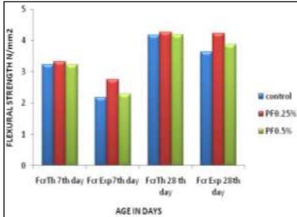
Figure 5: Flexural strength of PFRC at various ages
