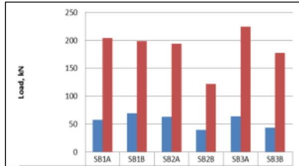
Figure 16: Initial and final crack loads
