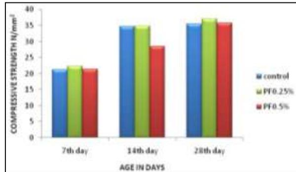
*Figure 3: Compressive strength of PFRC at various ages*
