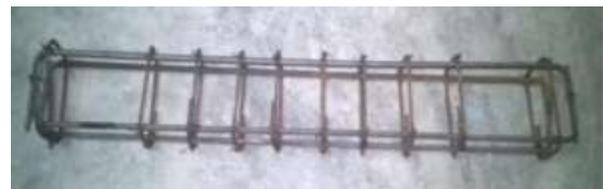
Figure 8: Reinforcement cage of shear beams
