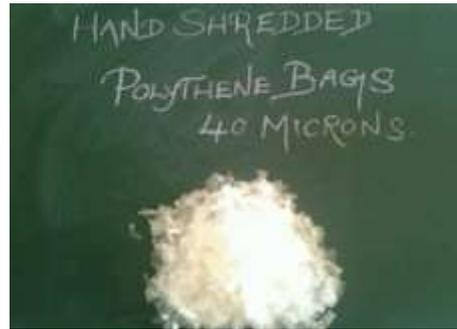
*Figure 1: Hand shredded PE bags of 40 microns*
