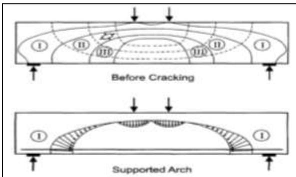
Figure 13: Internal arches in a RC beam [14]
