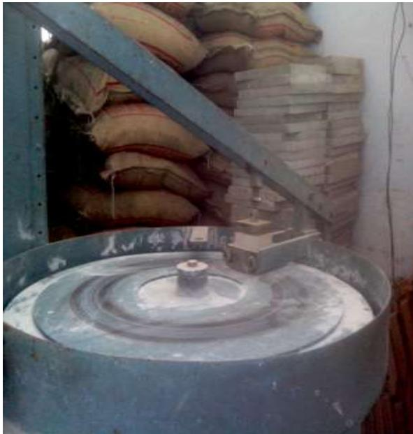
Figure 1: Abrasion Testing Machine
