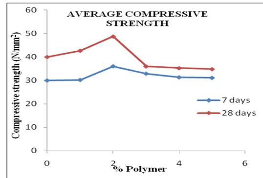
**Figure 2.1** Variation in average values of compressive strength for 7 days and 28 days
