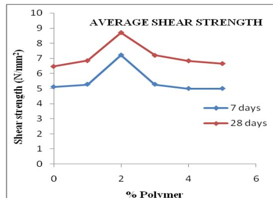
**Figure 2.2.** Variation in average values of shear strength for 7 days and 28 days
