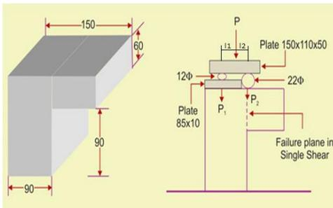
Figure 2.4 Shear Strength Test set-up as suggested by Bairagi and Modhera
