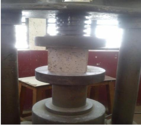
Figure 2.3 Compressive Strength Test set up
