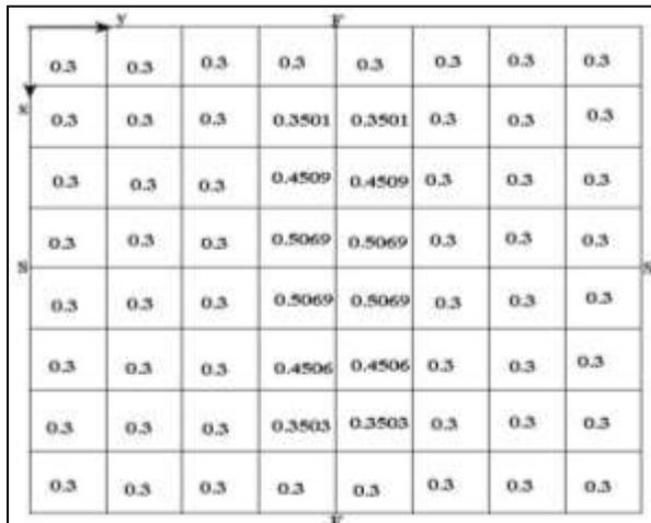
Figure 6 Element wise thickness distribution of shell under SFSF boundary condition (in mm)
