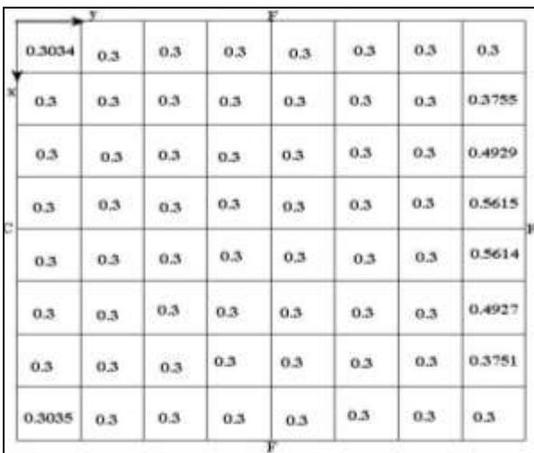
Figure 7 Element wise thickness distribution of shell under CFFF boundary condition (in mm)
