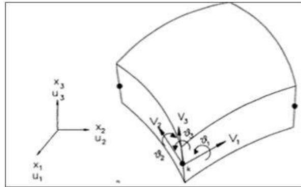
**Figure 2** Shell element showing unit vectors at mid plane of the shell
