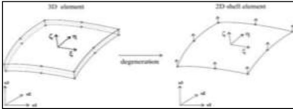
**Figure 1** Degeneration of a three dimensional shell element into a two dimensional element
