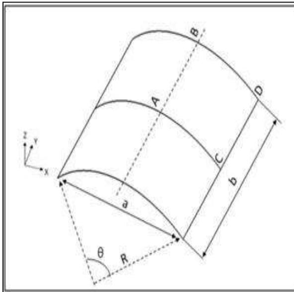
**Figure 4.** A typical shell geometry and its coordinate system
