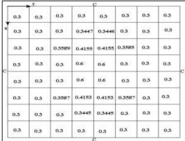
Figure 5 Element wise thickness distribution of shell under CCCC boundary condition (in mm)
