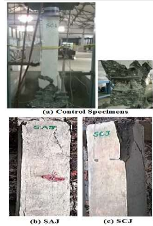
Figure 4 Failure patterns of control and retrofitted specimens
