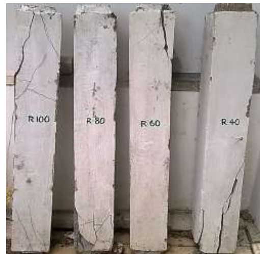
Figure 5 Failure patterns of rehabilitated specimens
