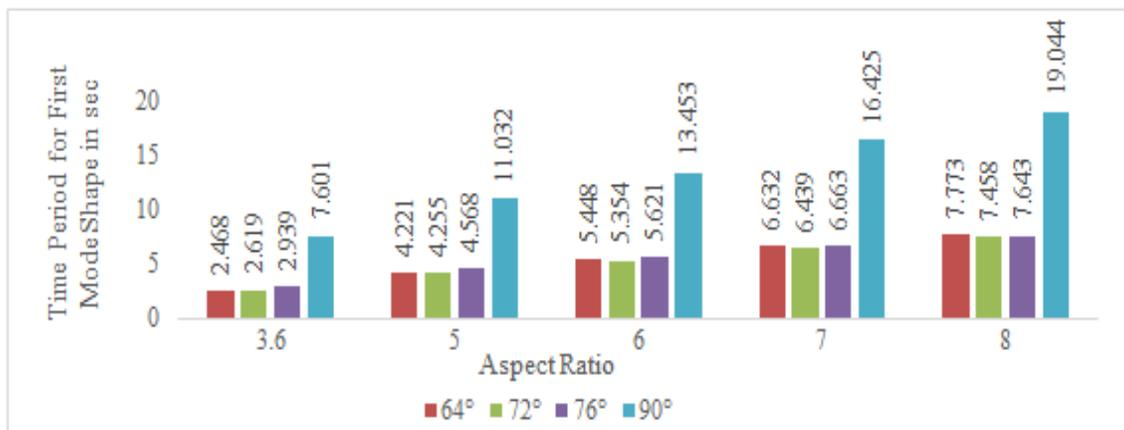
**Figure 8:** Time period for first mode shape for models of varying aspect ratio and varying angle of diagrid
