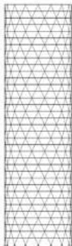
Figure 2: Diagonal columns inclined at 64.0°
