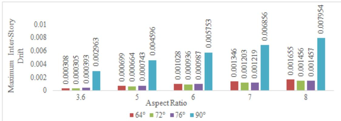
**Figure 7:** Maximum inter-storey drift for models of varying aspect ratio and varying angle of diagrid
