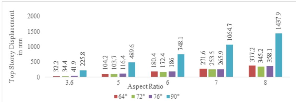
**Figure 6:** Top storey displacement for models of varying aspect ratio and varying angle of diagrid
