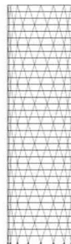
Figure 3: Diagonal columns inclined at 72.0°
