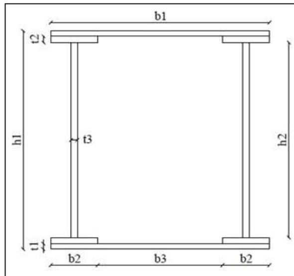
**Figure 10:** Typical Section of vertical column
