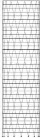
Figure 4: Diagonal columns inclined at 76.3°
