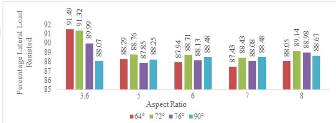
**Figure 9:** Lateral load resisted by diagrid by models of varying aspect ratio and varying angle of diaphragm
