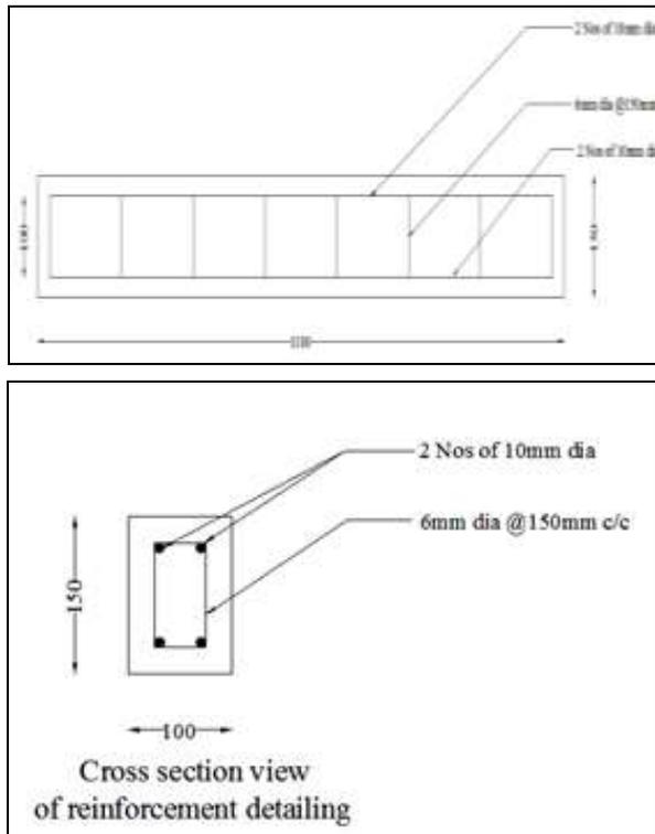
Fig 6.2.2 Reinforcement details
