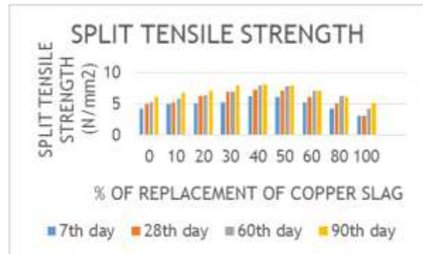
*Fig 6.2.1 Replacement % Vs Split Tensile Strength*
