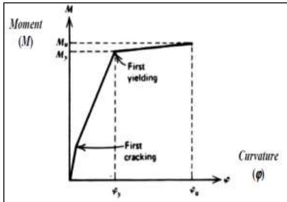
Fig.6.3.1 Trilinear moment-curvature relationship
