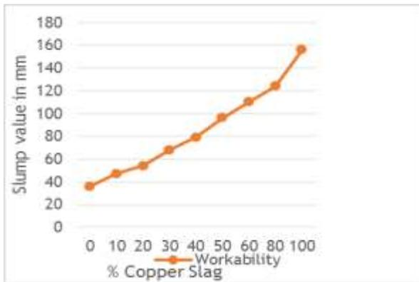
*Fig.5.1 Workability of concrete*
