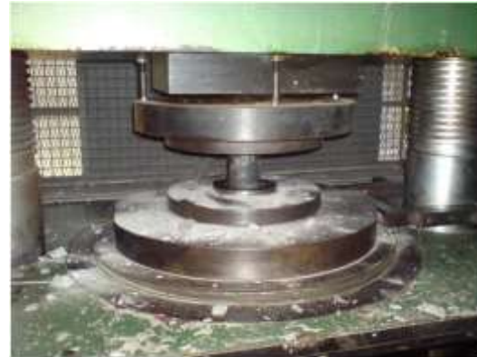
Figure 3 Testing of samples for UCS using 300 tonne compression testing machine
