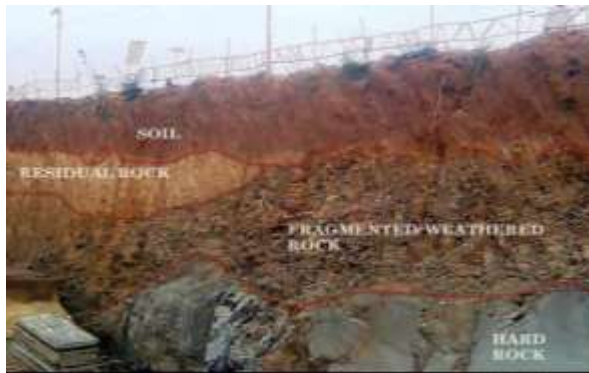
Figure 5 Classification of strata into soil, residual rock, weathered rock and hard rock
