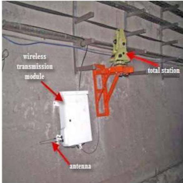
*Fig.9. Automatic monitoring system at tunnel sidewall*
