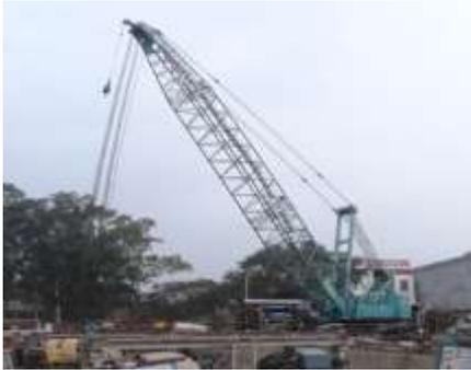
**Figure 3** 250 ton self-wt. crane
