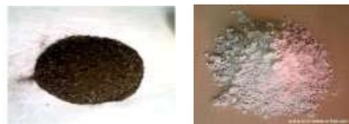
Figure 2 Ground granulated blast slag
