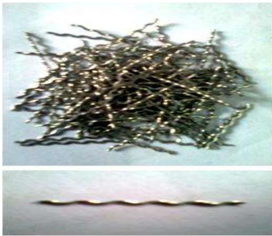
Figure 3 Crimped steel fibre
