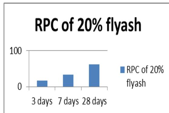
Figure 4 Compressive strength of RPC (flyash)
