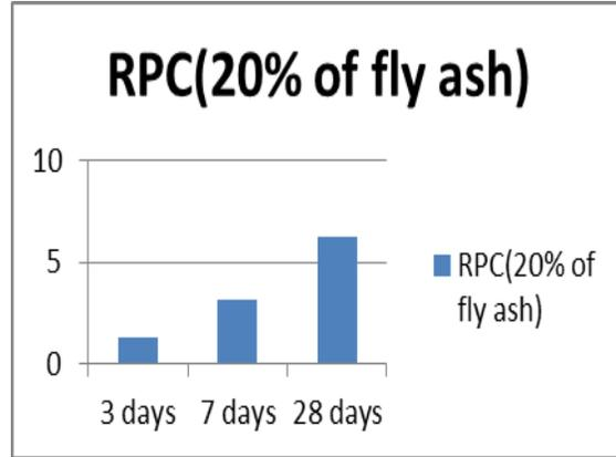
**Figure 6** Split tensile strength of RPC (flyash)
