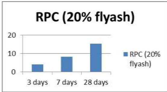
Figure 8 Flexural strength of RPC (20% flyash)
