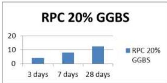
Figure 9 Flexural strength of RPC (GGBS)
