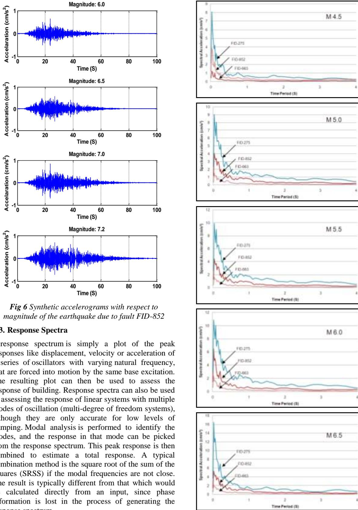
Fig 6 Synthetic accelerograms with respect to magnitude of the earthquake due to fault FID-852
