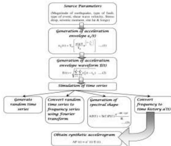
Fig. 4 flowchart of generation of synthetic accelerogram
