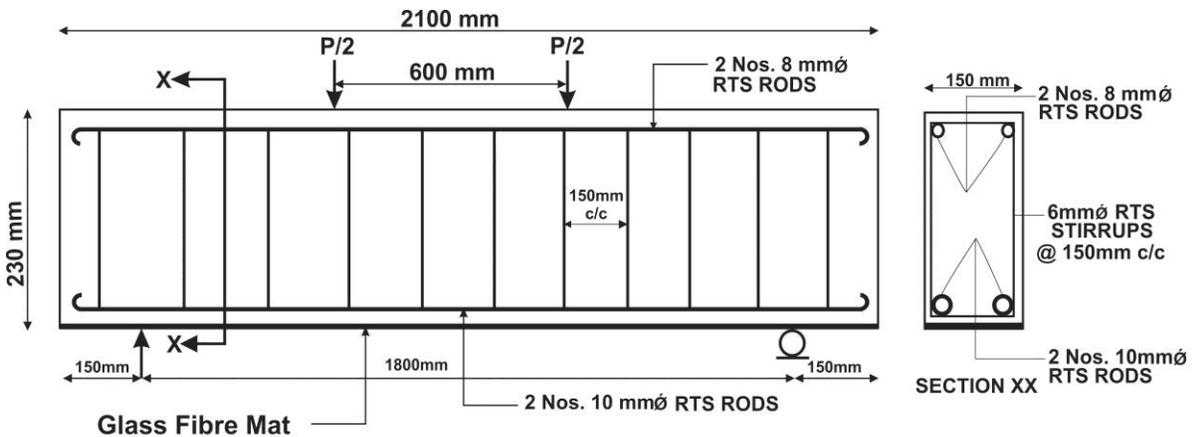
Figure 5 Section of Beam showing details of Reinforcement
