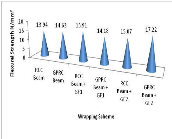
**Figure 7** Comparison of Average Flexural Strength of RCC and GPRC beams
