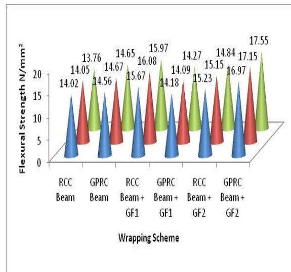
**Figure 6 Comparison of Flexural Strength of RCC and GPRC beams**
