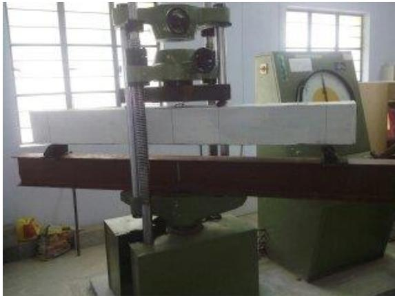
Figure 2 Experimental Setup - Beam with two points loading
