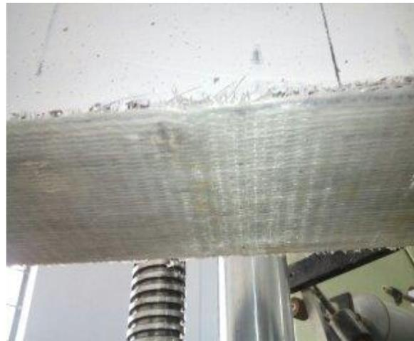
Figure 4 Beam with Glass fibre wrapped in tensile zone
