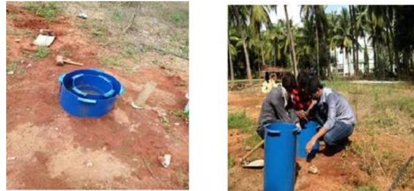
Fig 2: Doublring infiltrometer
