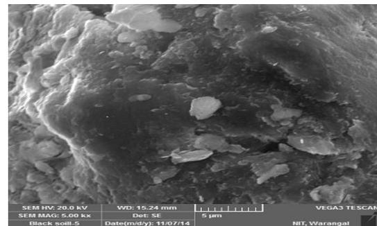
**Figure 1** SEM micrograph of uncontaminated black cotton soil
