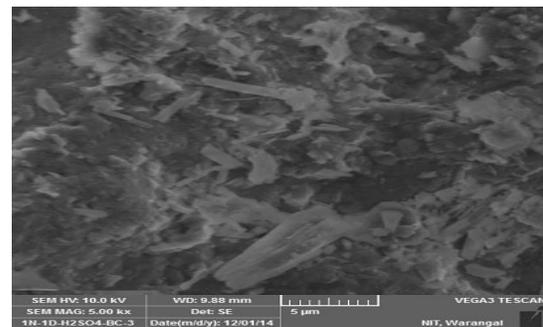
**Figure 2** SEM micrograph of black cotton soil contaminated with 1N  $\text{H}_2\text{SO}_4$
