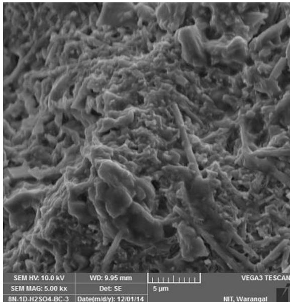
**Figure 4** SEM micrograph of black cotton soil contaminated with 8N H<sub>2</sub>SO<sub>4</sub>
