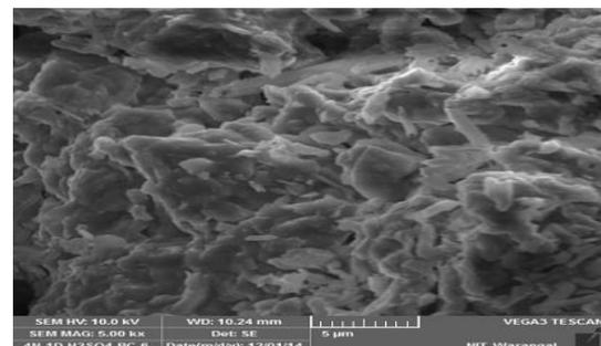
**Figure 3** SEM micrograph of black cotton soil contaminated with 4N H<sub>2</sub>SO<sub>4</sub>
