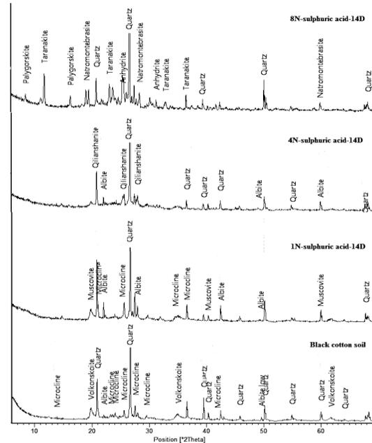
**Figure 6** X-ray diffraction patterns of black cotton soil before and after reaction with sulphuric acid of different concentrations for curing period of 14 days
