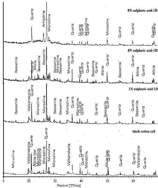
**Figure 5** X-ray diffraction patterns of black cotton soil before and after reaction with sulphuric acid of different concentrations for curing period of 1 day
