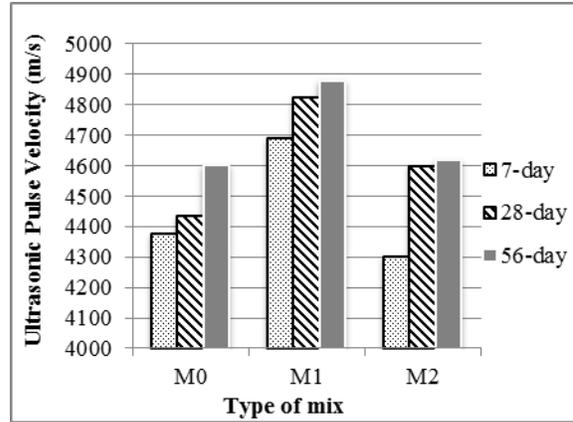
Figure 3. Ultrasonic pulse velocity of the concrete mixes
