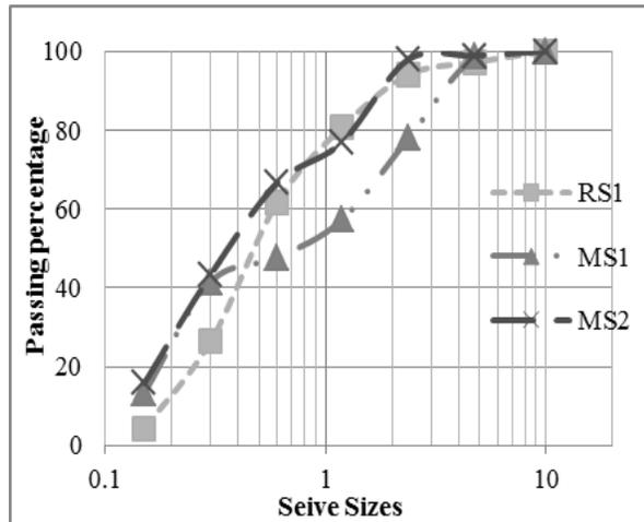
**Figure 1** Grading of fine aggregates
