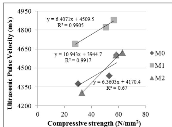
Figure 6 Variation in Ultrasonic pulse velocity with compressive strength
