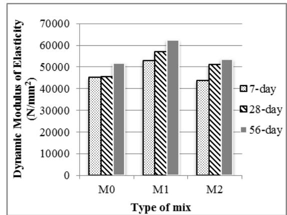
Figure 4 Dynamic Modulus of elasticity of the concrete mixes
