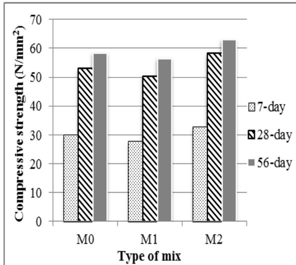
Figure 2. Compressive strength of the concrete mixes
