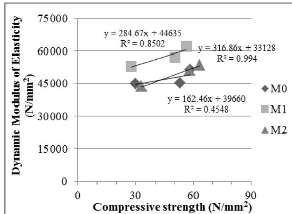
Figure 5 Variation in Dynamic modulus of elasticity with compressive strength
