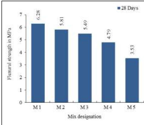
Figure 2 Flexural strength of SCC mixes at 28 days
