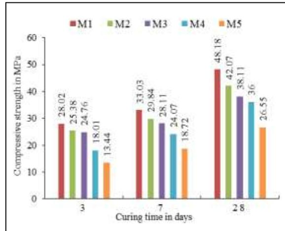
*Figure 1 Compressive strength of SCC mixes at different curing age*
