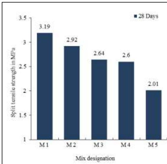
Figure 3 Split tensile strength of SCC mixes at 28 days
