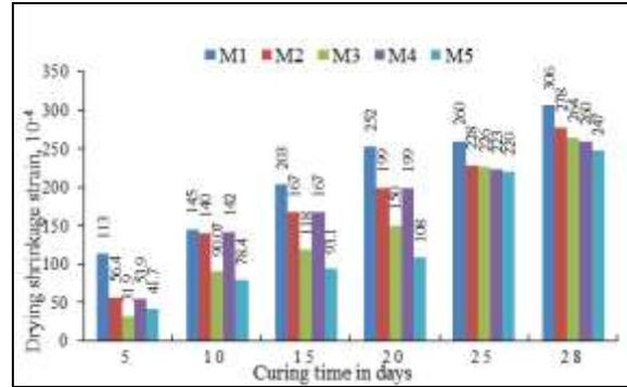
Figure 4 Drying shrinkage strain of SCC mixes at different curing age
