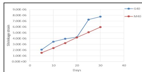
**Figure 3** Drying shrinkage strain for GPC and control mix
