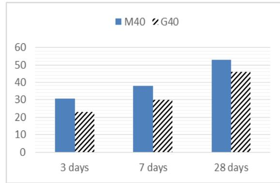
**Figure 1** Compressive strength for M40 and G40
