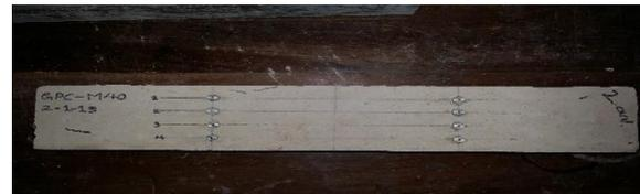
**Figure 2.** Buttons glued on the surface of the beam for measuring drying shrinkage
