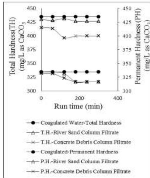
**Figure 6** Total Hardness (T.H.) and Permanent Hardness (P.H.) v/s Run time
