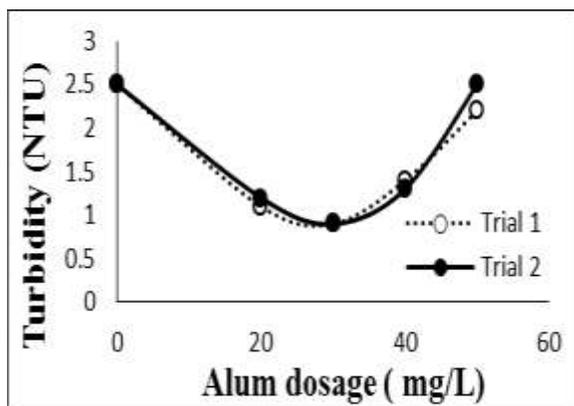
Figure 2 Turbidity v/s Alum dosage curve
