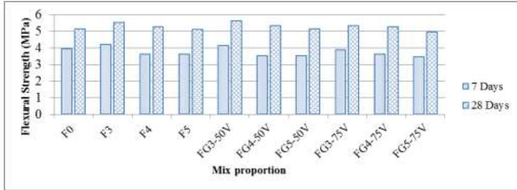
Figure 3 Flexural Strength at 7 days & 28 days
