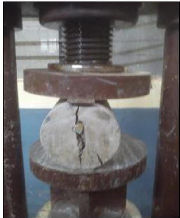
**Figure 4:** Test set up for split tensile test of concrete
