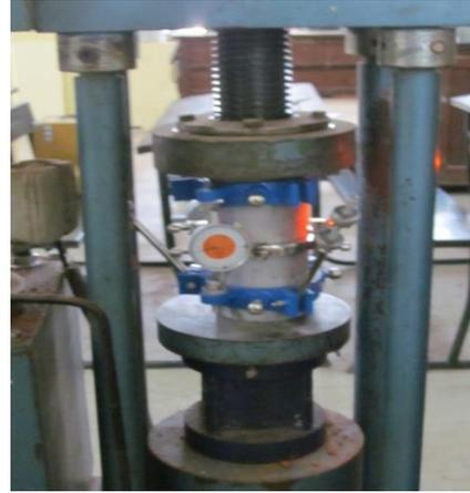
Figure 4: Experimental Test Setup for Modulus of Elasticity
