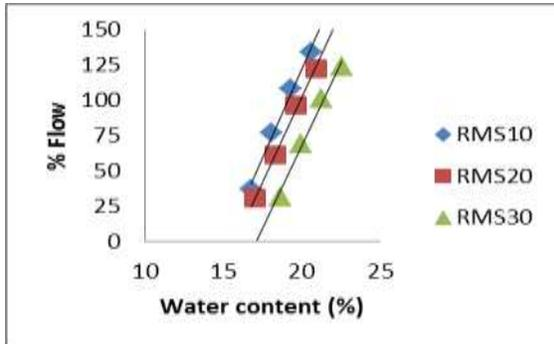
Figure 5 Flow versus total water content for reconstituted sands
