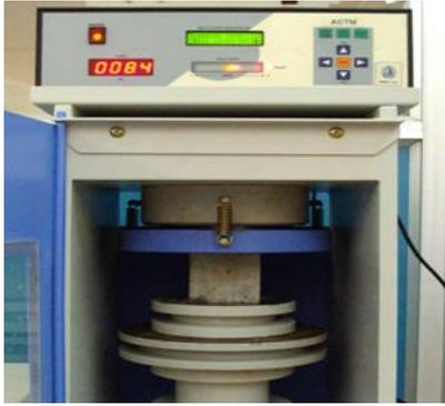
Figure 1: Cube compression test
