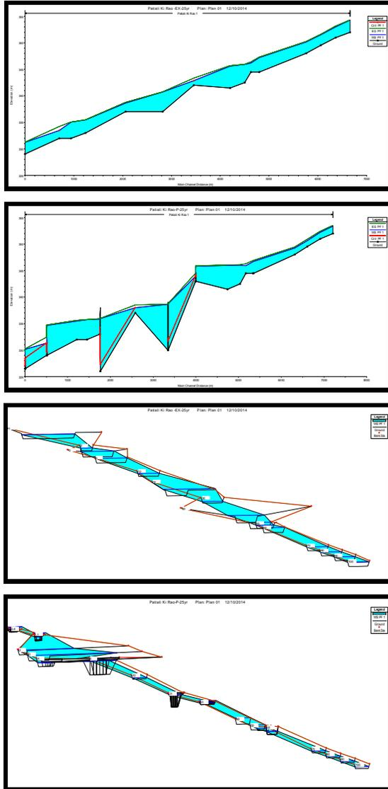
**Figure 3:** (a) Course of Patiali Rao from upstream to downstream during Existing condition; (b) Course of Patiali Rao from upstream to downstream during Present/Future Condition; (c) Plan View of Patiali Rao during Existing Condition and (d) Plan View of Patiali Rao during Present/Future Condition.
