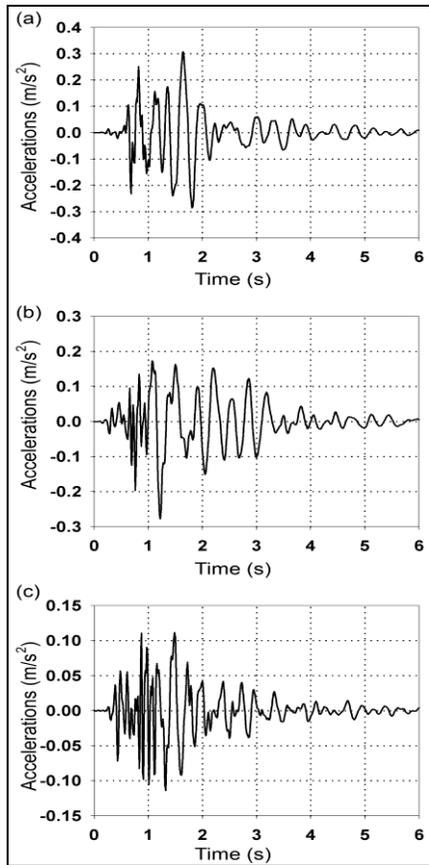
**Figure 1** Ground accelerations of the registered mining shock: a) in horizontal direction NS, b) in horizontal directions Y, c) in vertical direction Z
