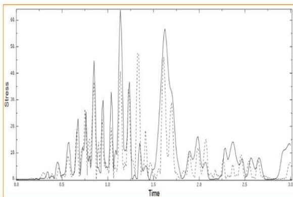
**Figure 5** Comparison of maximal principal stress obtained for: uniform (dashed line), non-uniform kinematic excitation (continuous line) at selected point 38609 (see Fig. 4)
