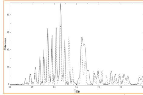
**Figure 6** Comparison of maximal principal stress obtained for: uniform (dashed line), non-uniform kinematic excitation (continuous line) at selected point 37724 (see Fig. 4)
