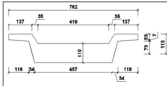
**Figure 2** Dimensions of the cross section of the viaduct deck in the middle of the main span
