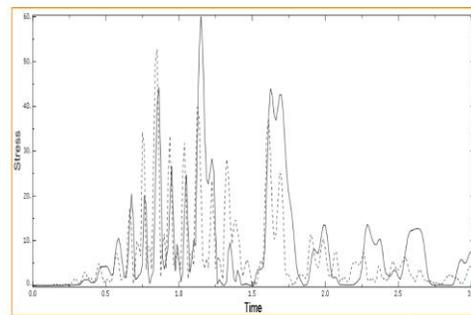
**Figure 7** Comparison of maximal principal stress obtained for: uniform (dashed line), non-uniform kinematic excitation (continuous line) at selected point 38900 (see Fig. 4)
