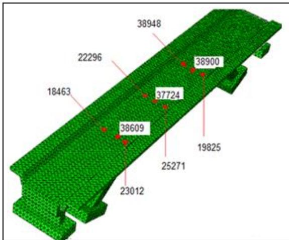
**Figure 4** FE mesh along with the location of points selected for dynamic analysis
