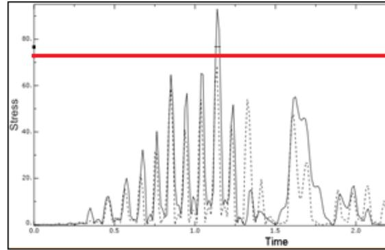
**Figure 9** Maximal principal stress obtained with THA method for uniform (dashed line) and non-uniform excitation (continuous line) as well as with the RSA method (red line) at point 37724
