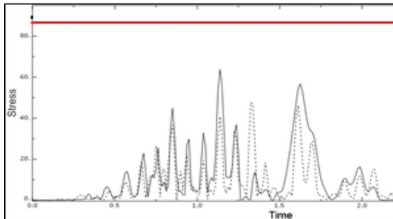
**Figure 8** Maximal principal stress obtained with THA method for uniform (dashed line) and non-uniform excitation (continuous line) as well as with the RSA method (red line) at point 38609
