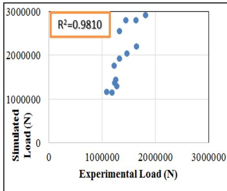
Figure 8 Comparison of Experimental Load values for Validation Set
