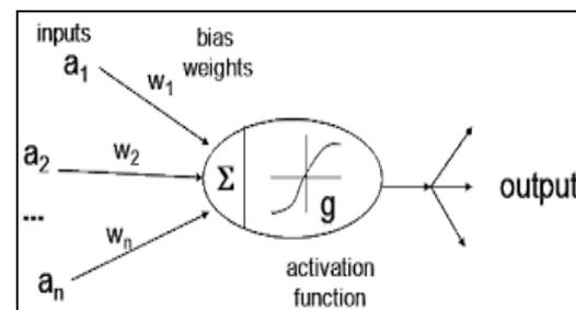
**Figure 2** Schematic Computation of Neuron
