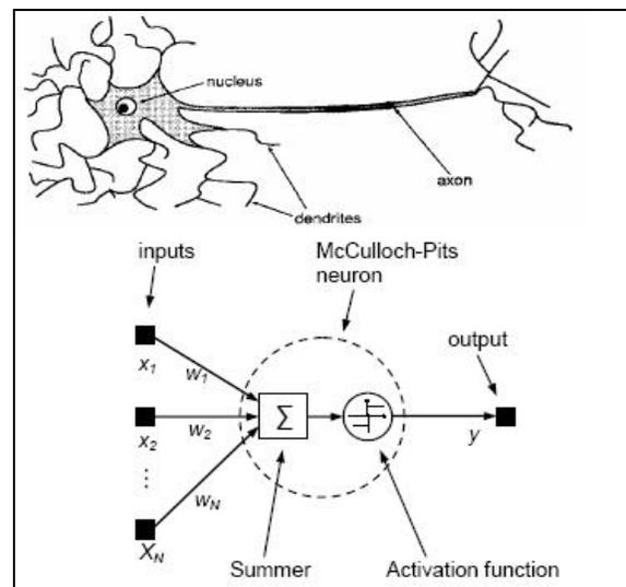
**Figure 1** A biological neuron model, which processes  $N$  inputs ( $xN$ ) to arrive at the output ( $y$ ).
