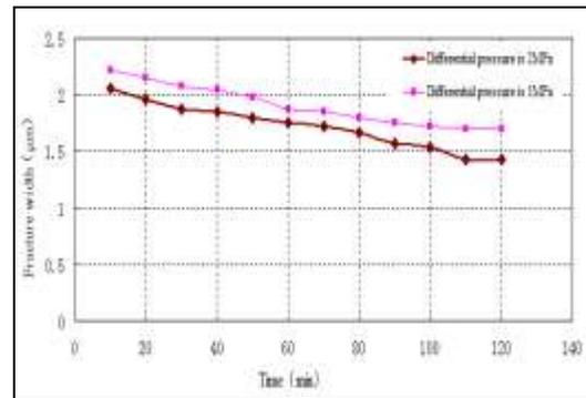
**Fig7:** Fracture width curve with the test time changes under the different test pressure
