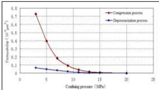
**Fig1: Stress sensitivity curve of QS1# coal rock**
