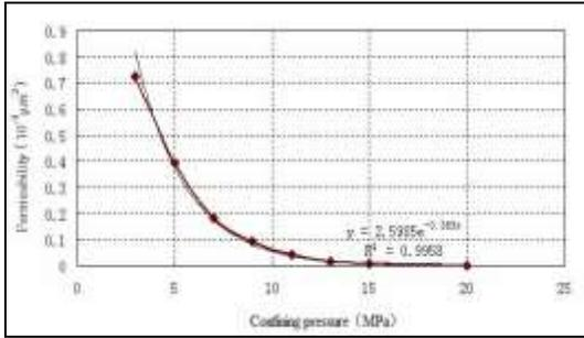
**Fig3:** Fitting curve of QS1# coal rock between Permeability and net confining pressure
