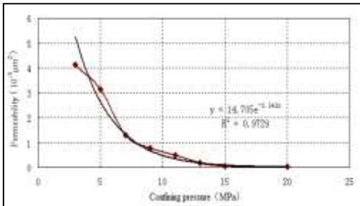
**Fig4:** Fitting curve of QS2# coal rock between Permeability and net confining pressure
