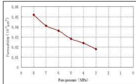
**Fig5:** Pore pressure sensitivity curve of coal and rock
