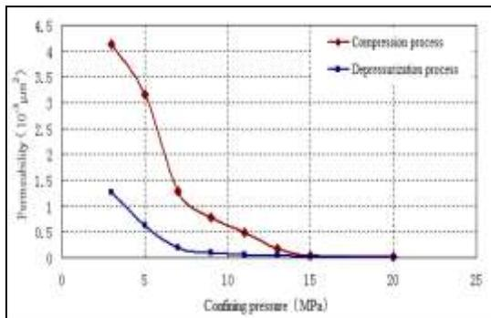
**Fig2: Stress sensitivity curve of QS2# coal rock**
