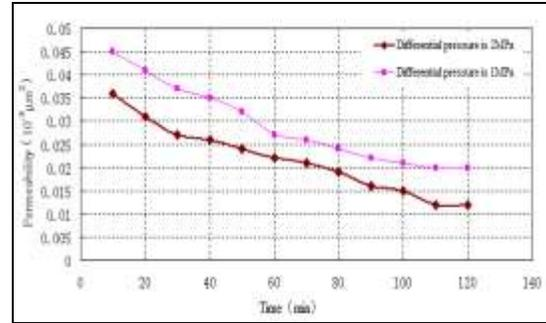
**Fig6:** Permeability curve with the test time changes under the different test pressure
